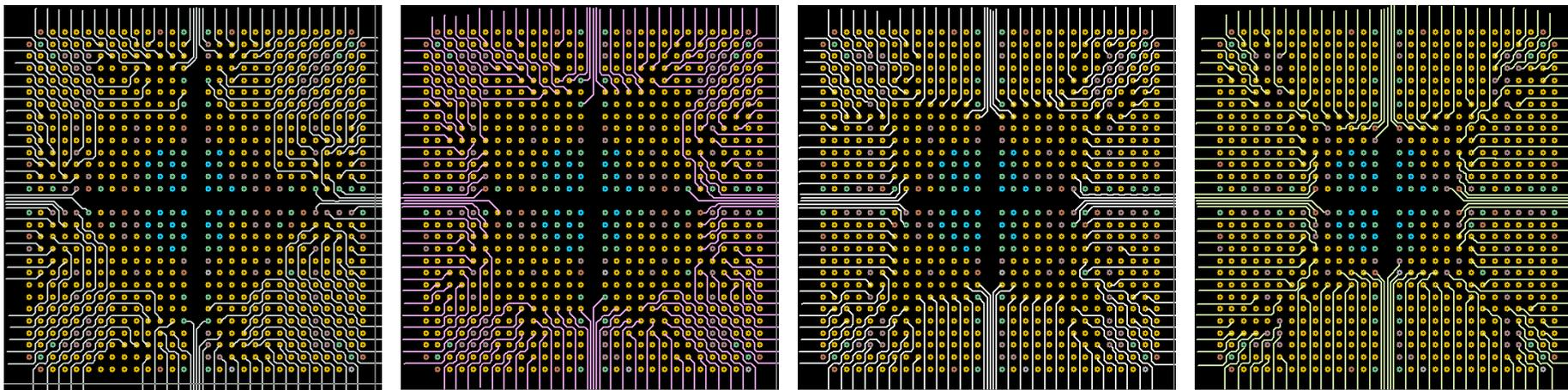
Notice the 45 degree routing required to utilize the corners. Also 5 between in “plus sign/cross”.
